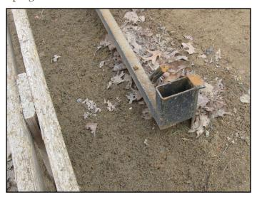
These tubes are designed to accept a common 2x4 to support a steel target. Members need only bring their 4' long 2x4 and (conforming) steel target, set it in the receiving tube, and they are good to go. Sure beats carrying a target stand back and forth from home to the target area.
