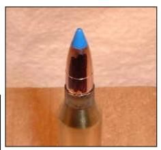
Now measure from that line to the base of the loaded cartridge. This is your optimum "Base to Bore" dimension for that rifle. It will be valid for almost ANY bullet, no matter what nose profile. If you change bullets, simply mark the new bullet with the same scribed line, using your calipers, and seat it to the same Base to Bore distance. The new bullet will then be the same "off lands" distance as your first bullet.
