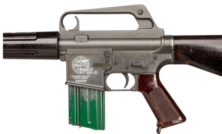
Left side closeup of ArmaLite prototype AR-15 S/N 000001. Note the AR-10 trigger type charging handle.
