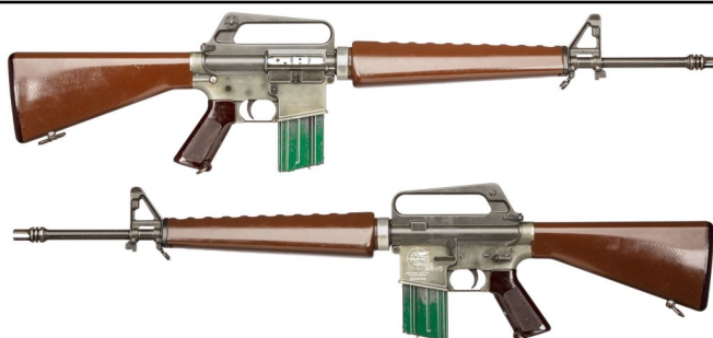
Left and right-side view of ArmaLite prototype AR-15 S/N 000004. A 601-type upper receiver group from a later phase of the development of the AR-15 has been paired with the S/N 000004 lower despite the fact that it was first built during an earlier phase.
