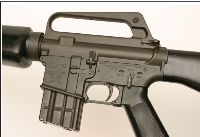
Left side closeup of COLT/ArmaLite AR-15 Model 601 S/N 001081. The rifle's original green painted furniture has been replaced by black painted furniture. Photo by the author
